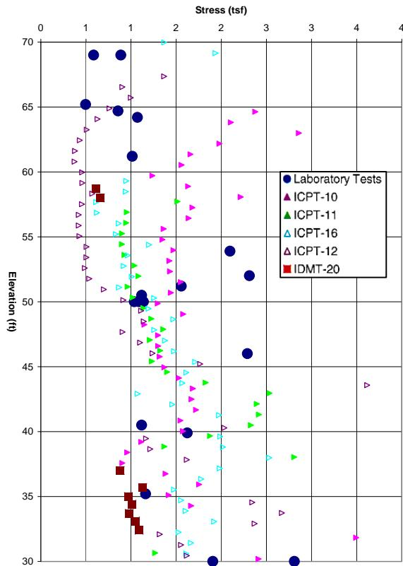
Figure 2a. IDMT-17 Undrained Shear Strength
