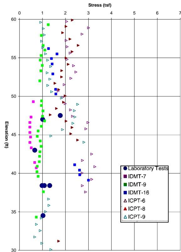
Figure 2c. IDMT-7, 9 &amp; 16 - Undrained Shear Strength
