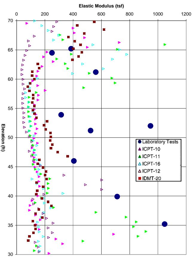
Figure 4b. IDMT-20 Tangent Modulus,  $E_i$  and DMT Modulus  $E_D$
