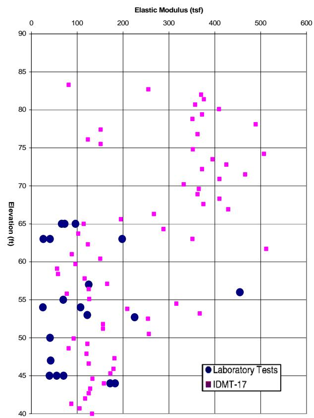
Figure 4a. IDMT-17 Tangent Modulus,  $E_i$  and DMT Modulus  $E_D$
